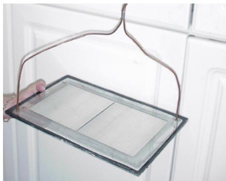
Solar cell mock-up to examine the WVTR of edge sealant material
